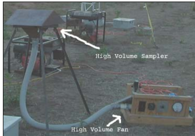
Figure 4.7. High Volume Sampling Setup.
