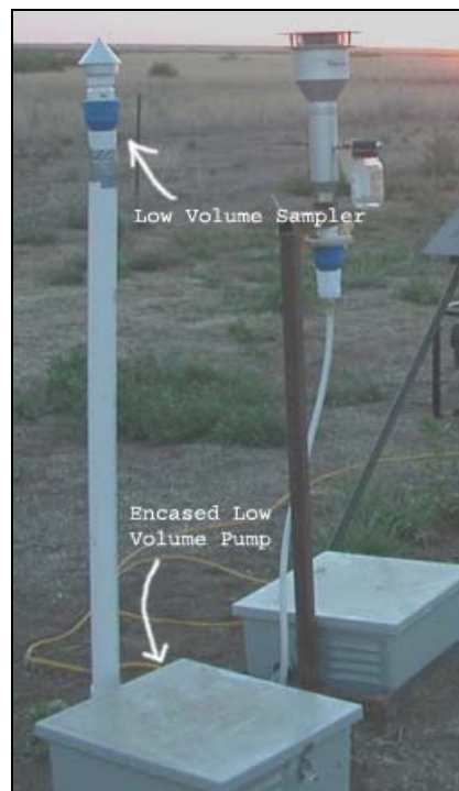
Figure 4.8. Low Volume Sampling Setup.
