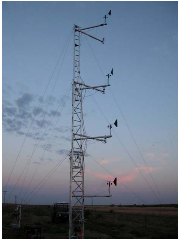
Figure 5.1. Tower with Co-located Anemometers and Receptors.
