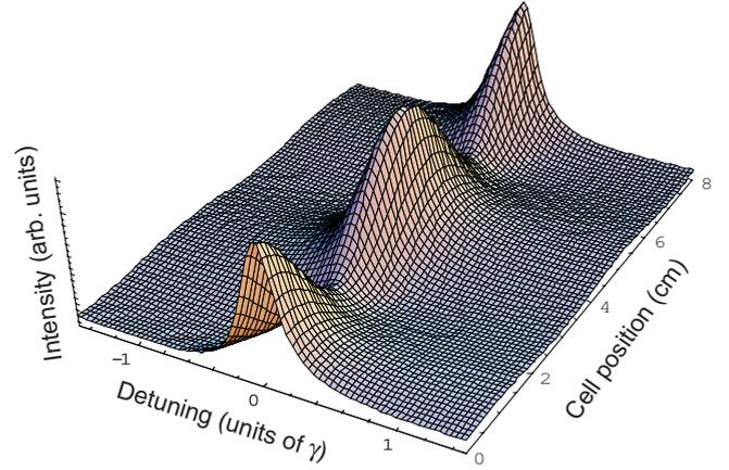
FIG. 7. (Color online) Numerical simulation of the transmission of the probe field dependence on detuning and cell positions. In the simulation, we use  $\gamma_{ab}=5$ ,  $\gamma_{bc}=10^{-3}$ ,  $\Omega_{10}=0.1$ ,  $\Omega_2=1$ ,  $\Omega_\mu=0.02$ ,  $\eta=0.9$ ,  $L=2.5$  cm, and  $\Delta k=1.5$   $\text{cm}^{-1}$ .
