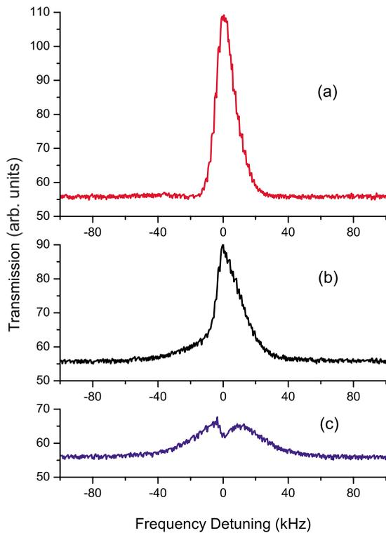
FIG. 3. (Color online) The beating signal recorded by a spectrum analyzer at the center frequency of 7.035 GHz. It represents the transmission of the probe field. (a) The enhanced transmission with the microwave field applied; (b) the transmission without the microwave field applied; (c) the suppressed transmission with the microwave field applied. The positions of the cell where (a) and (c) were taken are about 2.2 cm apart.
