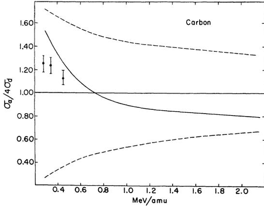
FIG. 1. Comparison of theoretical calculation for  $r_{12}$  with experimental data taken from Ref. 2 for  $\alpha$  and deuteron bombardment of carbon.
