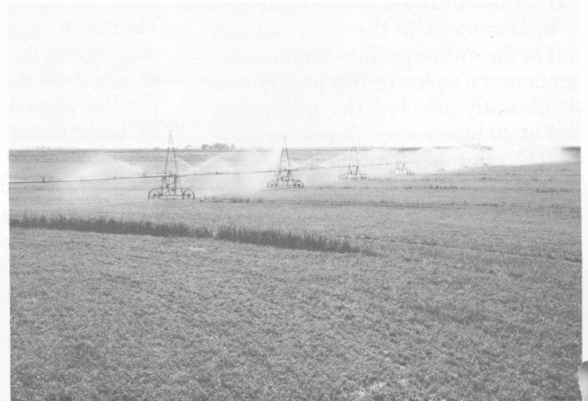
Fig. 14. Irrigating alfalfa in Parmer County, Texas, with a high-pressure, center pivot sprinkler system (USDA — Soil Conservation Service photo).
