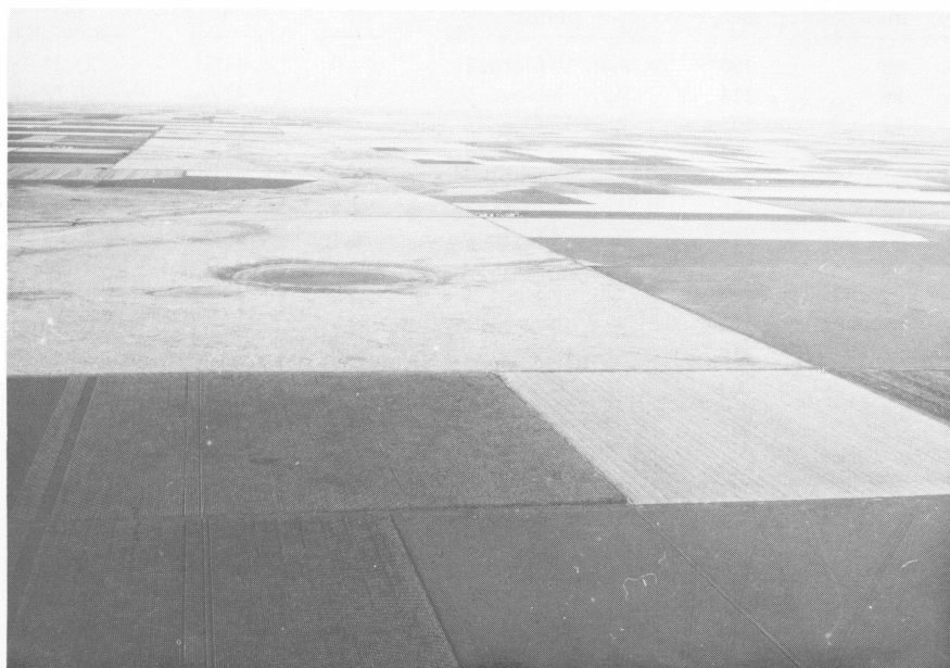
Fig. 4. Aerial view of the topography of the land occupied by Pullman soils. The circular area near the center is a playa, or shallow lake, which contains other soils (USDA — Soil Conservation Service photo).
