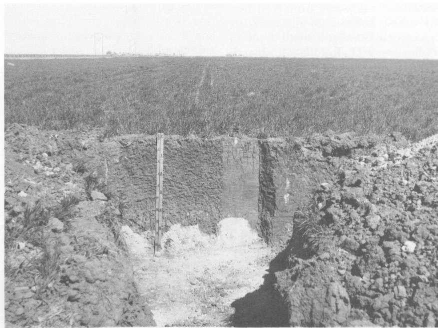
Fig. 9. Surface conditions and soil profile at a typical site of Pullman soil. The site is at the USDA Conservation and Production Research Laboratory, Bushland, Texas (USDA — Soil Conservation Service photo).
