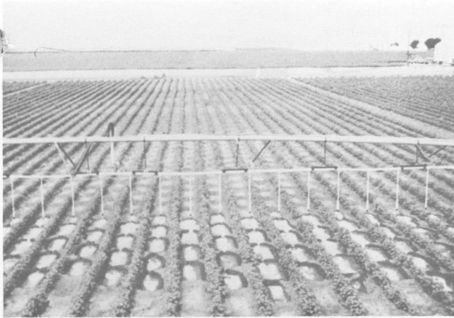
Fig. 15. Experimental low pressure sprinkler being used on a furrow-blocked field (Photo provided by W. M. Lyle, TAES).
