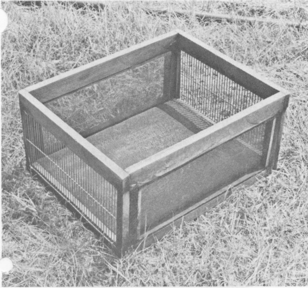
Fig. 9. Basket type grader.
