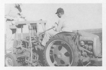
Figure 26B: Small self-propelled nursery harvester designed at Texas Substation No. 6, Denton, Texas.
