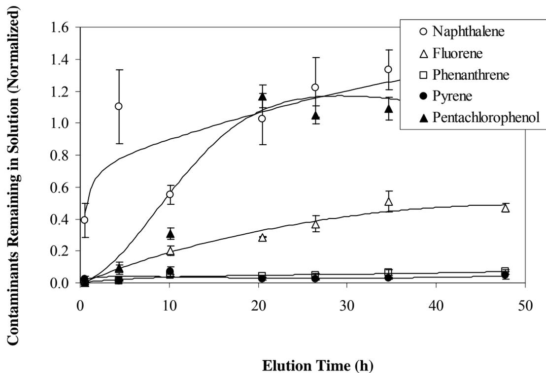
Figure 24. Contaminants remaining in solution at selected time points over 48 h of continuous elution of OWS effluent through 3:2 CP-LPHM/GAC. Values represent mean concentrations for 3 separate composite columns (normalized to untreated OWS effluent)  $\pm$  SE.
