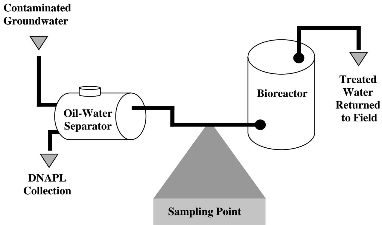
Figure 20. Schematic representation of the groundwater treatment facility used for field research. Groundwater from the aquifer is pumped into the oil-water separator (OWS) (10,000 gal). After separation, DNAPL is removed. The aqueous phase is routed to two, parallel, fixed-film bioreactors (10,000 gal each) and then applied to on-site land treatment units.
