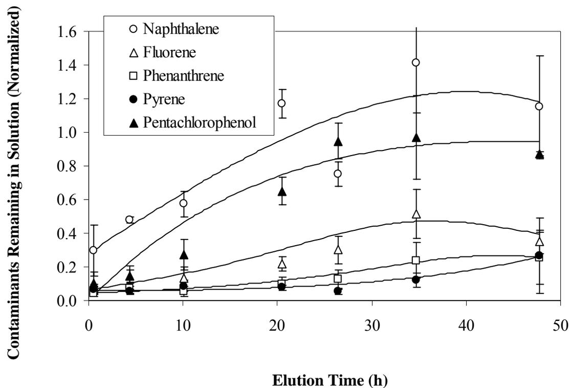
Figure 25. Contaminants remaining in solution at selected time points over 48 h of continuous elution of OWS effluent through CP-LPHM/sand. Values represent mean concentrations for 3 separate composite columns (normalized to untreated OWS effluent)  $\pm$  SE.
