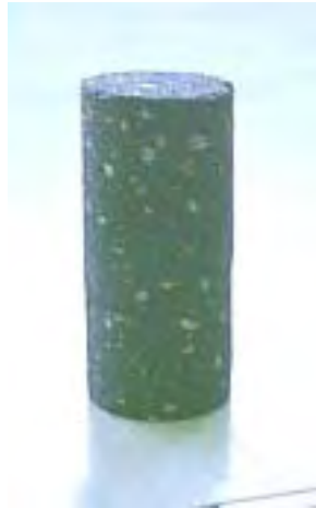
Fig. 2. Test Specimen After Coring
