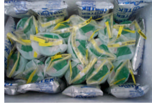
C: samples were surrounded by 10 360-ml ice refrigerants
