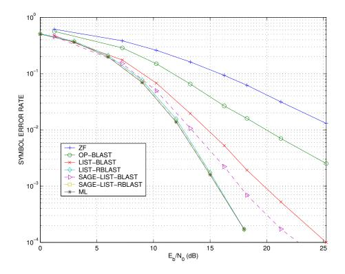
Fig. 14. Symbol Error Rate of different detectors for a  $4 \times 4$  MIMO system with uncoded 8-PSK modulation.
