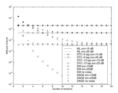
Fig. 25. The convergence of MSE with respect to number of iterations of the EM-type estimators compared with the MSE of a 9-tap-STC, 13-tap-STC estimator and the ML estimator. An initial channel estimate is obtained using (7.25). The uniform profile as shown in (a) of Fig. 22 is assumed.
