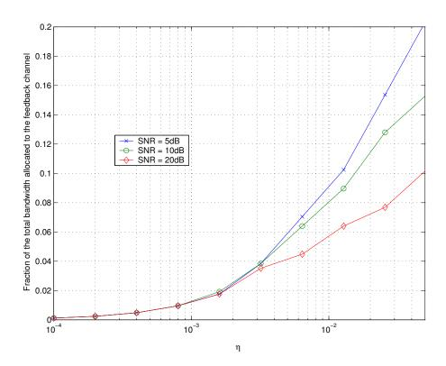
Fig. 12. Optimal fraction of the total bandwidth allocated to the feedback channel for different  $\eta$  in order to achieve  $C_d^*$ .  $N_t=4$ .
