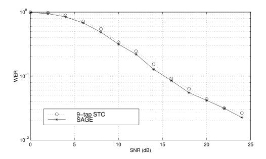
Fig. 28. BER and WER of ST-OFDM system for channels with the HT profile as shown in (b) of Fig. 22.
