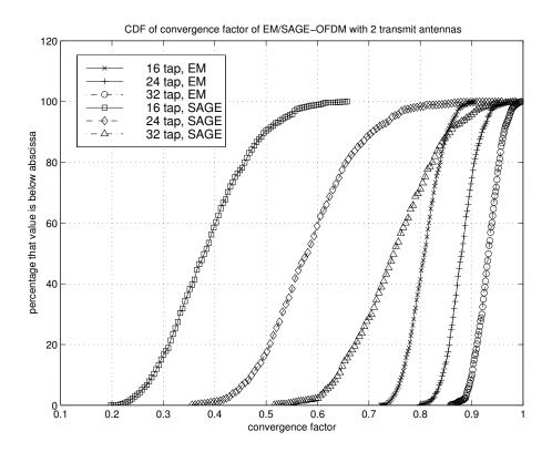
Fig. 26. CDF of convergence factor of EM-type estimators with two transmit antennas used.
