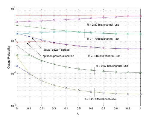
Fig. 8. Minimum outage probability achievable by optimal and equal power allocation over the directions indicated by the two eigenvectors of covariance matrix  $\Sigma$ . Note that the two eigenvalues,  $\lambda_1$  and  $\lambda_2$  satisfy  $\lambda_1 + \lambda_2 = 2$ . Channel received SNR, SNR<sub>rv</sub>  $\stackrel{\triangle}{=} \frac{P}{\sigma_n^2}$ , is fixed at 8dB.
