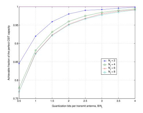
Fig. 9. The random quantization lower bound to the achievable rate for the beamforming scheme vs  $\frac{B}{N_t}$  for different  $N_t$ . Channel SNR, defined as  $\frac{P\sigma_h^2}{\sigma_n^2}$ , is fixed at 10 dB.
