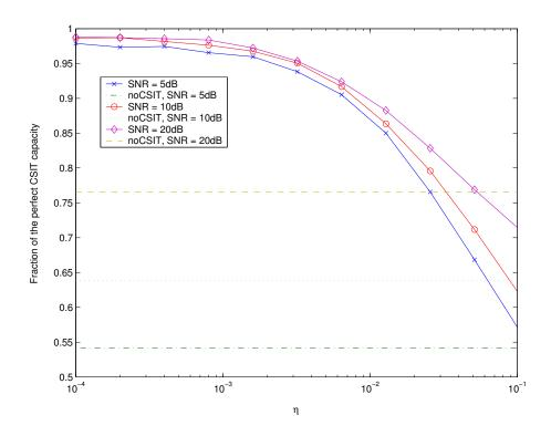
Fig. 11. Maximum achievable rate  $C_d^*$ , normalized by the capacity with perfect CSIT obtained using the random quantization lower-bound for different  $\eta$ .  $N_t = 4$ .
