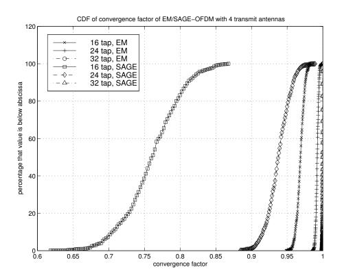
Fig. 27. CDF of convergence factor of EM-type estimators with four transmit antennas used.
