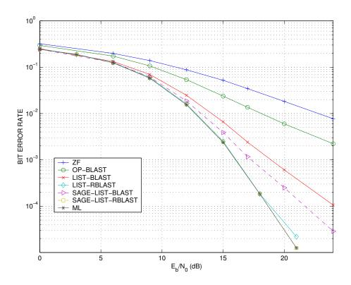
Fig. 17. Bit Error Rate of different detectors for a  $4\times4$  MIMO system with uncoded 16-QAM modulation.
