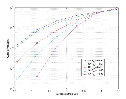
Fig. 5. Achievable minimum outage probability vs target rate of mean-feedback for  $N_t=2$ . Channel received SNR, SNR<sub>rv</sub>  $\stackrel{\triangle}{=} \frac{P(\xi+\sigma_h^2)}{\sigma_n^2}$ , is fixed at 8dB. SNR<sub>fb</sub>  $\stackrel{\triangle}{=} \frac{\xi}{\sigma_h^2}$ .
