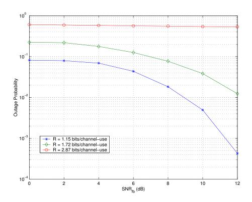
Fig. 6. Effect of  $\mathrm{SNR}_{fb}$  on achievable minimum outage probability of mean-feedback for  $N_t=2$ . Channel received  $\mathrm{SNR}$ ,  $\mathrm{SNR}_{rv} \stackrel{\triangle}{=} \frac{P(\xi+\sigma_h^2)}{\sigma_n^2}$ , is fixed at 8dB.  $\mathrm{SNR}_{fb} \stackrel{\triangle}{=} \frac{\xi}{\sigma_h^2}$ .
