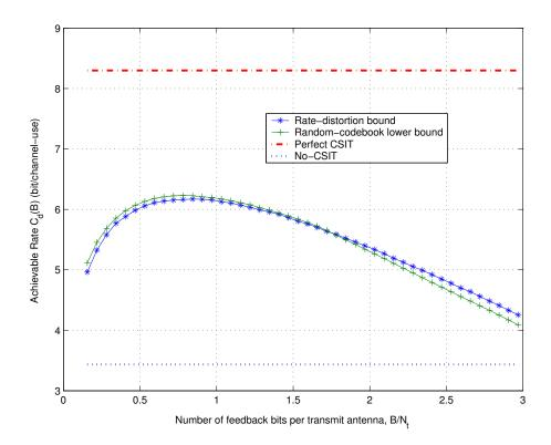
Fig. 13. Comparison of achievable rates assuming two different partial CSIT models:  $N_t=32$  ,  $\eta=0.005$  and SNR = 10 dB.
