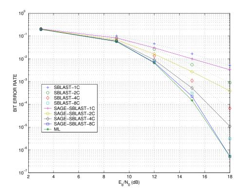
Fig. 18. Bit Error Rate of different detectors for a  $8 \times 8$  MIMO system with uncoded 16-QAM modulation.
