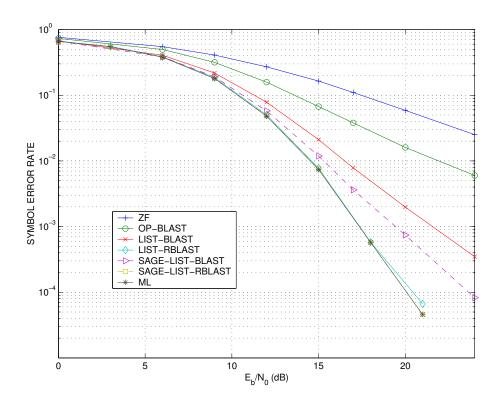
Fig. 16. Symbol Error Rate of different detectors for a  $4\times4$  MIMO system with uncoded 16-QAM modulation.
