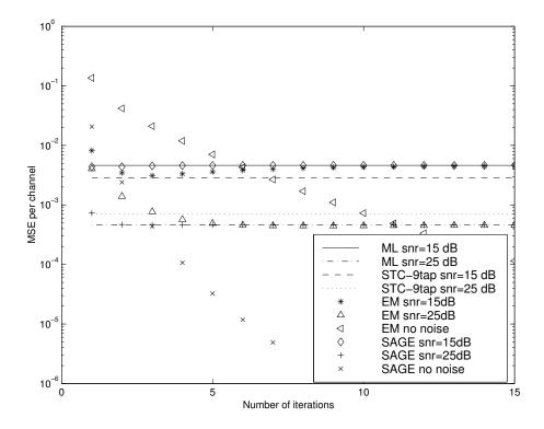
Fig. 24. The convergence of MSE with respect to number of iterations of the EM-type estimators compared with the MSE of a 9-tap-STC estimator and the ML estimator. The EM algorithm is initialized using the last channel estimate. The HT profile as shown in (b) of Fig. 22 is assumed.
