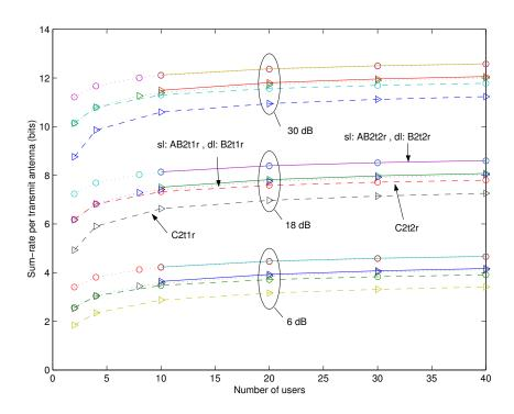
Fig. 1. Upper-bounds on sum-rate capacity for  $N_t=2$ . ("Bxtyr", "ABxtyr" and "Cxtyr" denote capacity bound (equation (3.13)), asymptotic bound (equation (3.20)), and sum-rate capacity with  $N_t=x$  and  $N_r=y$ , respectively; "sl" and "dl" denote solid line and dotted line, respectively.
