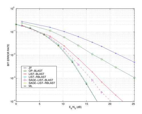
Fig. 15. Bit Error Rate of different detectors for a  $4\times 4$  MIMO system with uncoded 8-PSK modulation.
