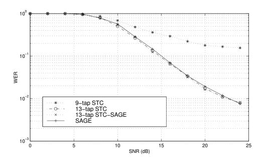
Fig. 29. BER and WER of ST-OFDM system for channels with the uniform profile as shown in (a) of Fig. 22.
