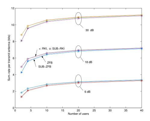
Fig. 4. Achievable sum-rate per transmit antenna for different user selection criteria  $(N_t = 2)$ .
