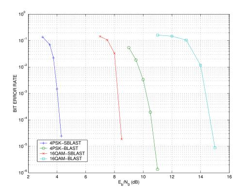
Fig. 19. Bit Error Rate of turbo-coded  $4 \times 4$  MIMO systems with SAGE-aided List-Shifted-BLAST decoding and the simple soft-output BLAST decoding.
