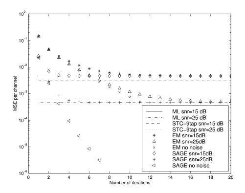
Fig. 23. The convergence of MSE with respect to number of iterations of the EM-type estimators compared with the MSE of a 9-tap-STC estimator and the ML estimator. An initial channel estimate is obtained using (7.25). The HT profile as shown in (b) of Fig. 22 is assumed.
