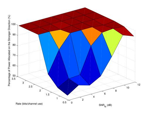
Fig. 7. Optimal power allocation over different transmission directions of mean-feedback for  $N_t=2$ . Channel received SNR,  $\mathrm{SNR}_{rv} \stackrel{\triangle}{=} \frac{P(\xi+\sigma_h^2)}{\sigma_n^2}$ , is fixed at 8dB.  $\mathrm{SNR}_{fb} \stackrel{\triangle}{=} \frac{\xi}{\sigma_h^2}$ .
