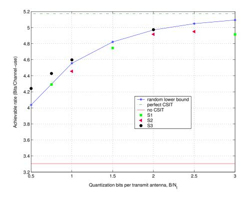
Fig. 10. Achievable rates of practical quantization schemes for  $N_t = 4$  and SNR=10dB.
