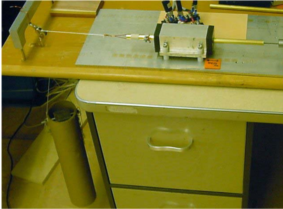
Figure 5-1: Experimental setup to determine maximum pullout force. The load hangs from a string that is held by the motor via a pulley. Load is incrementally increased to the hanging mass by adding small weights.
