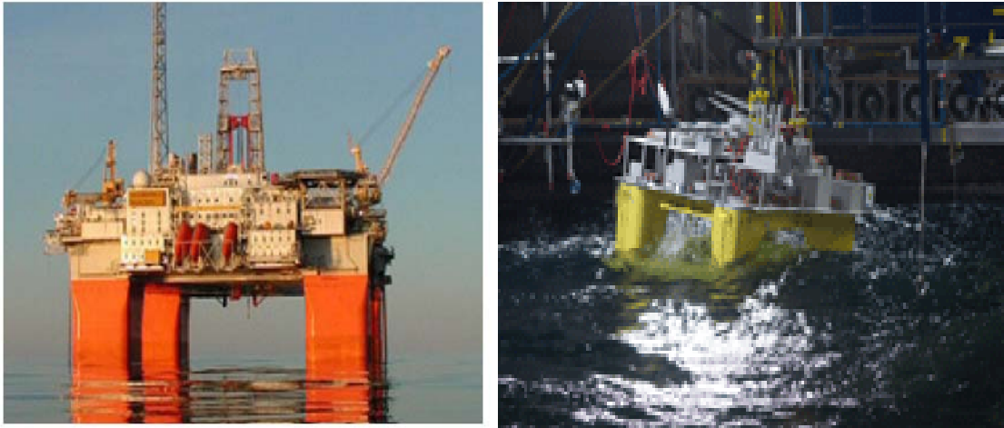
Fig. 1.3: Discrepancies between full depth floater and model scale floater Source: Experimental methods in marine hydrodynamics (NTNU) [2]
