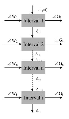
Figure 3.7. Cascade diagram for mass integration (El-Halwagi, 2006)
