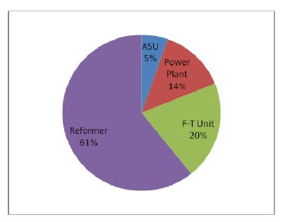
Figure 1.7. CO<sub>2</sub> from each unit (Iandoli and Kjelstrup, 2007)
