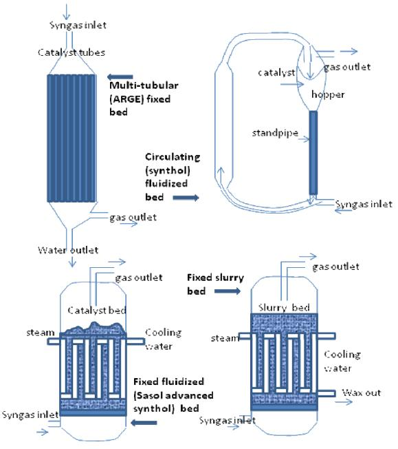
Figure 1.5. F-T reactors (Spath and Dayton, 2003)
