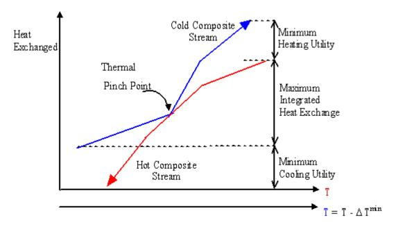
Figure 3.9. Thermal pinch diagram (El-Halwagi, 2006)
