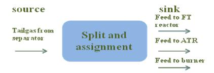
Figure 5.9. Assignment of split fractions and assignment to sinks for GTL process
