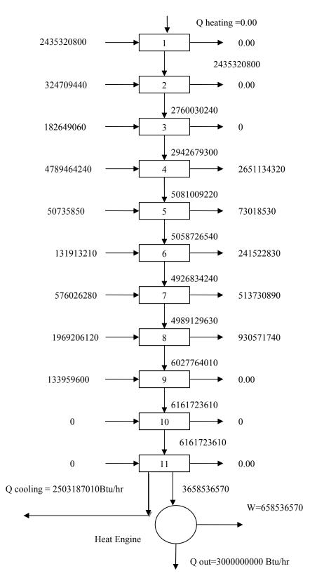
Figure 5.6. Integrating of the heat engine with HEN
