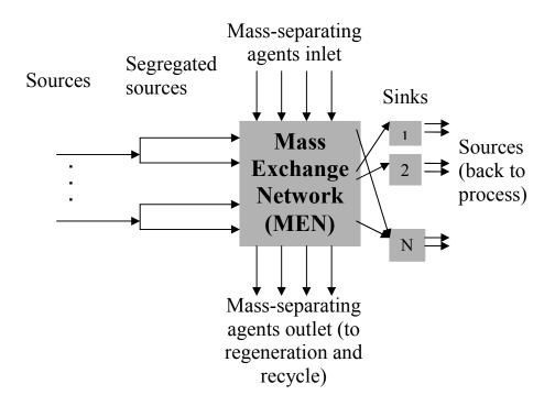
Figure 3.5. Process from species perspective when integrated (El-Halwagi, 2006)
