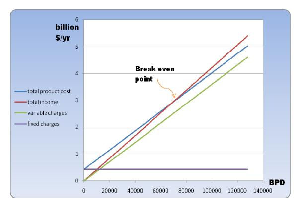
Figure 5.13. Break-even point calculation
