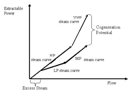
Figure 3.15. Extractable power cogeneration targeting pinch diagram (El-Halwagi, 2006)
