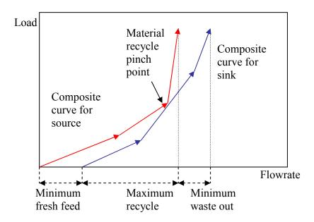
Figure 3.6. Identifying pinch point for maximum recycling (El-Halwagi, 2006)
