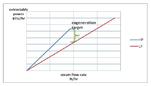
Figure 5.7. Unshifted extractable power versus flowrate plot
