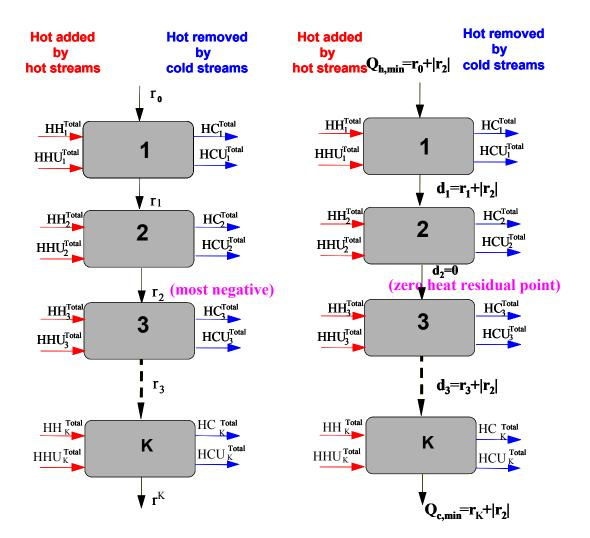
Figure 3.12. Cascade diagram for HENs (El-Halwagi, 2006)
