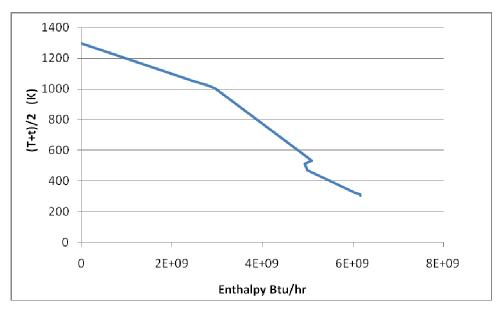
Figure 5.5. Grand composite curve for the GTL process
