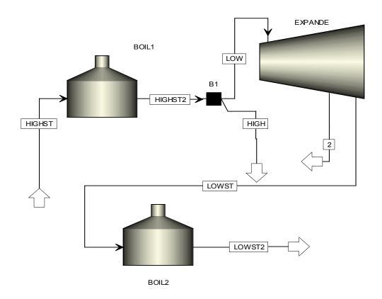
Figure 5.8. Representation of the cogeneration flowsheet
