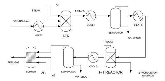
Figure 4.1. Schematic representation of the base-case GTL flowsheet
