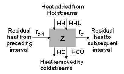
Figure 3.11. Heat balance around a temperature interval (El-Halwagi, 2006)
