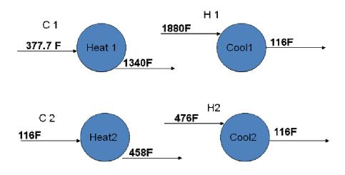
Figure 5.2. Description of the hot and cold streams
