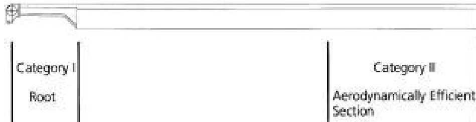
Figure 2. There are two control concept categories: Category I applies control forces at the root, Category II applies control forces near the blade tip [1].
