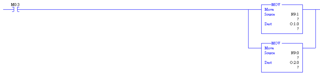
Figure 22 An example PLC rung on read/write Register
