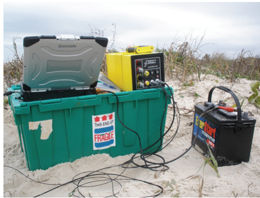
Fig. 4.1. Field setup of equipment. A car battery powers the console and data is collected with Toughbook laptop
