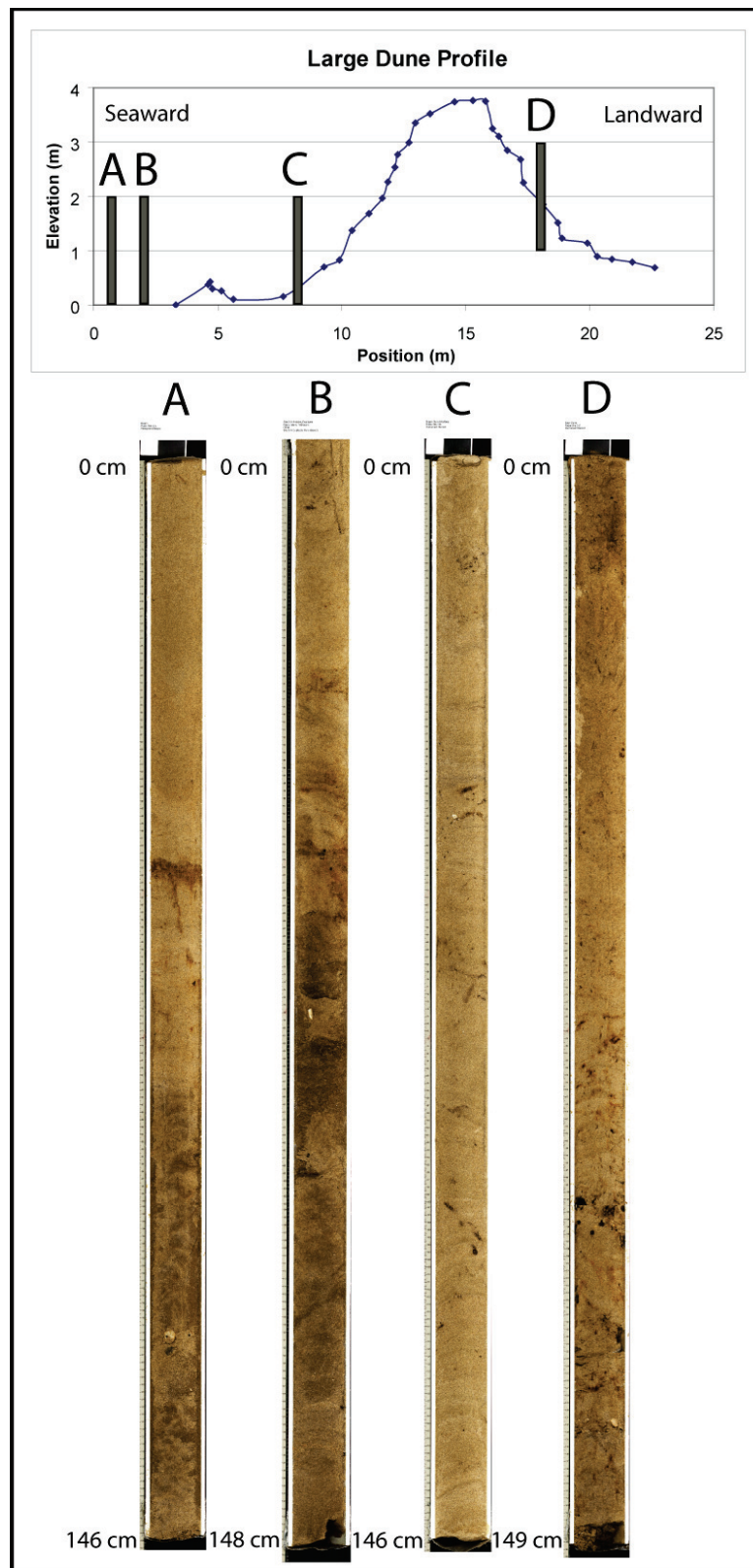
Fig. 5.2. Diagram of the cores taken at Site 3 [Weymer, 2014].
