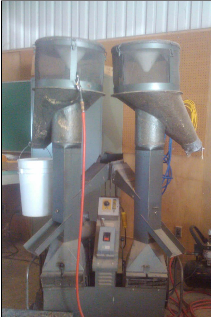
Fig. 10. Erie Magnetics seed blower used to separate seed from debris.
