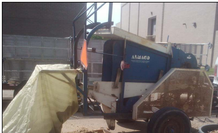
Fig. 9. Almaco thresher used to separate sunflower seed from the heads.
