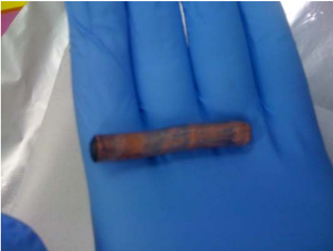
Figure (4-2) – The fully extruded portion of the sample measured two inches long and a quarter inch in diameter.
