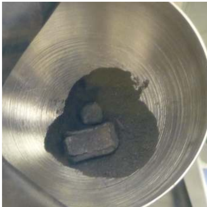
Figure (3-4) – Example of uranium powder product prior to classification via sieving [4].
