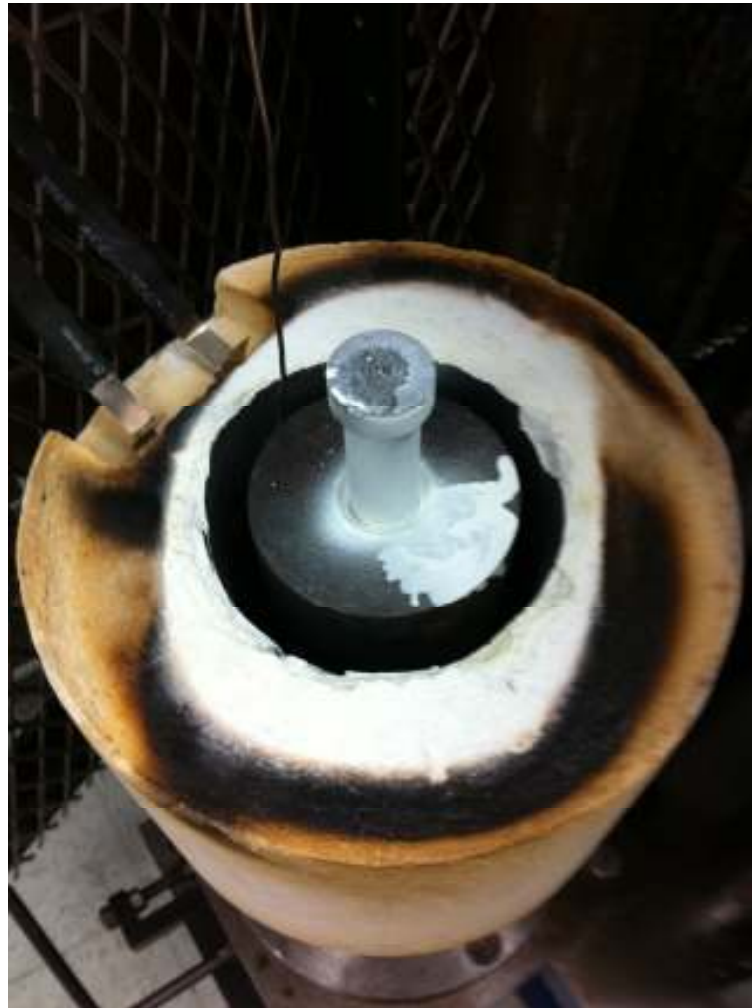
Figure (3-9) – View of the extrusion assembly during heating. The white coating is boron nitride lubricant, to decrease resistance due to friction.
