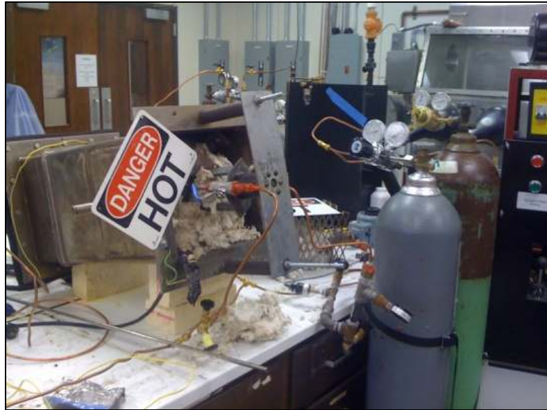
Figure (3-2) – Larger hydride-dehydride reaction system adapted from R.D. Kelley's zirconium hydride experiment.
