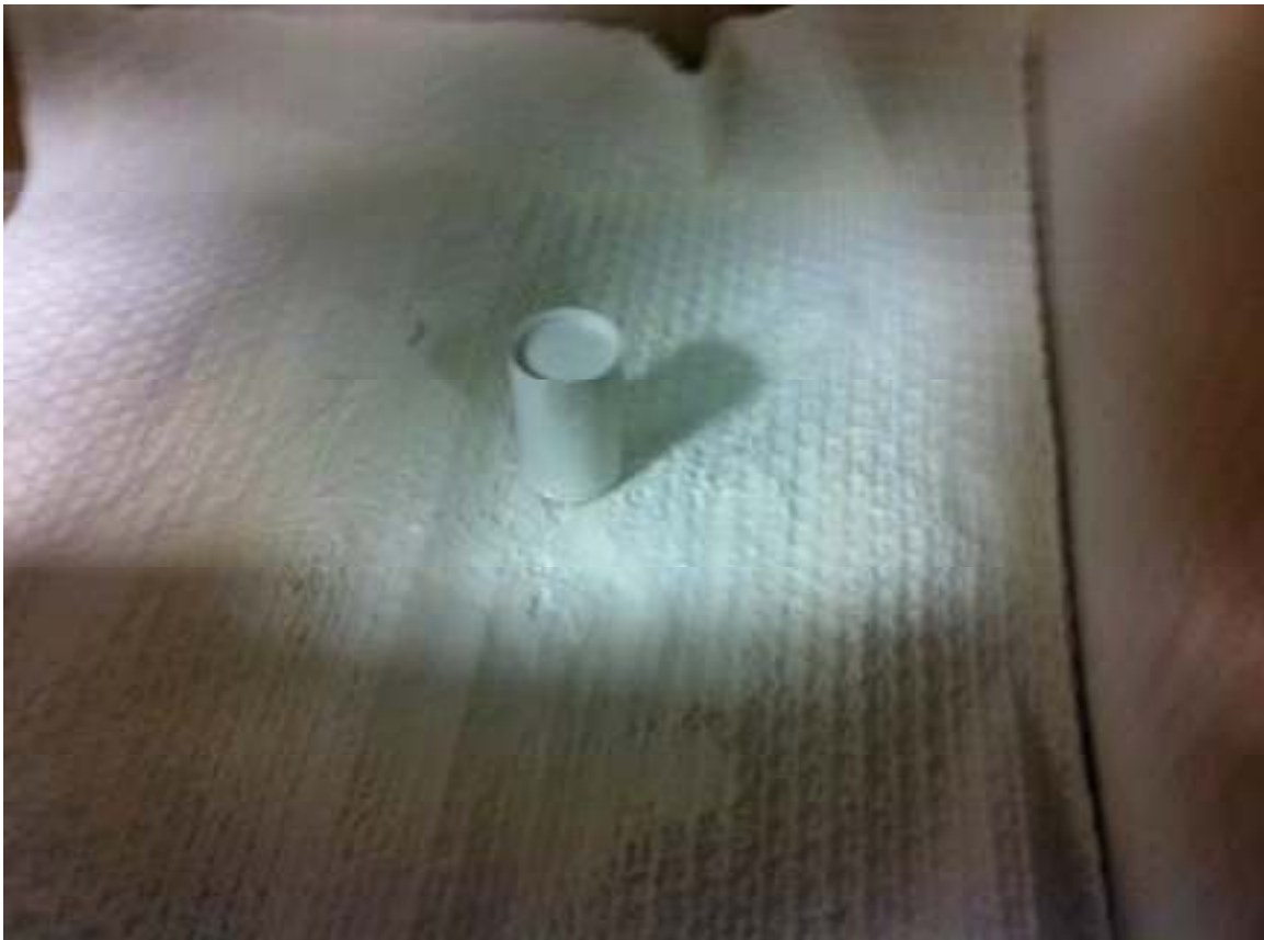
Figure (3-6) – The sealed sample canister after coating with boron nitride.
