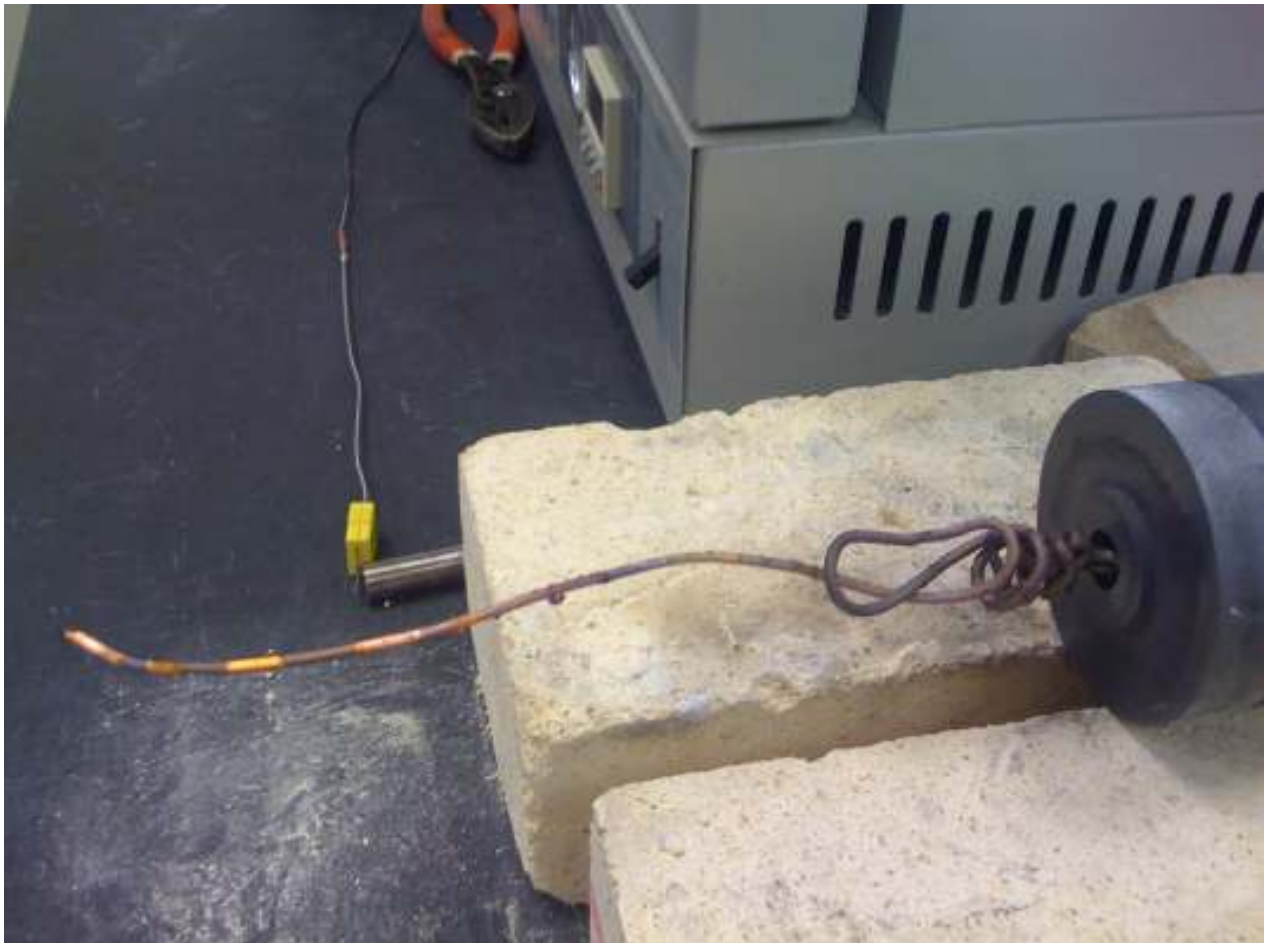
Figure (4-1) – The remains of the copper plug after the extrusion.
