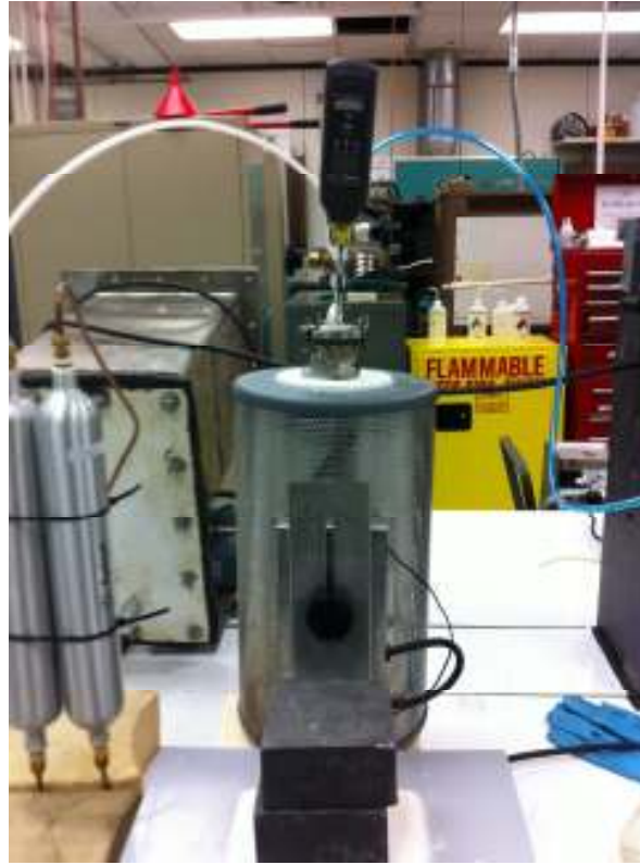
Figure (3-3) –Larger-scale hydride-dehydride apparatus developed to produce powder for extrusion experiments.
