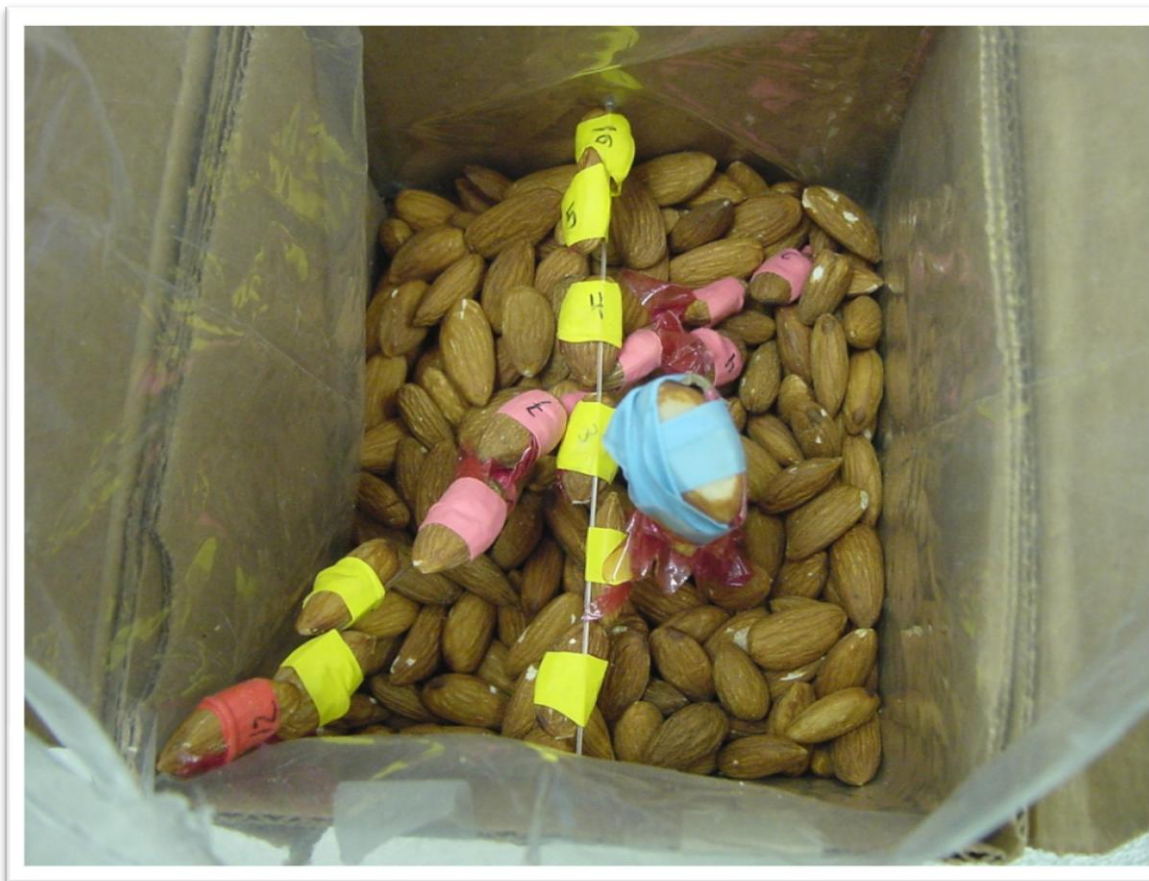
Figure 3-Alanine dosimeters fixed in a horizontal, vertical and diagonal configuration inside a 12.7 x 12.7 x 12.7 cm cardboard box filled with almonds.
