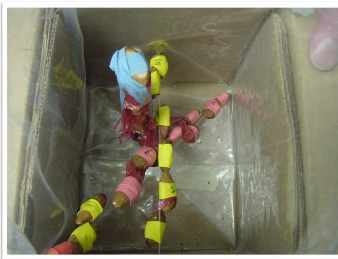
Figure 2-Alanine dosimeters fixed in a horizontal, vertical and diagonal configuration inside a 12.7 x 12.7 x 12.7 cm cardboard box.
