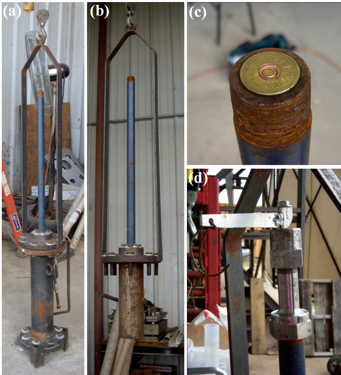
Figure C-1. Shock tube apparatus. (a) Entire apparatus, (b) barrel and cone, (c) shotgun shell loaded in barrel, (d) firing mechanism.
