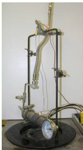
Figure A-1. Very-short-term pretreatment reactor.
