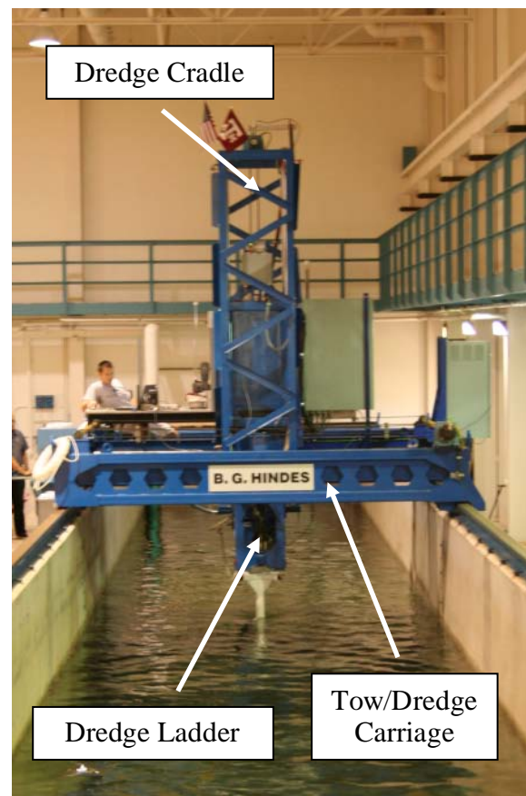
Figure 12. Towing/Dredge Carriage During Typical Anchor Towing Test.
