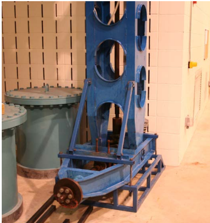
Figure 13. Articulating Arm and Lower Section of Dredge Ladder on Storage Cradle.
