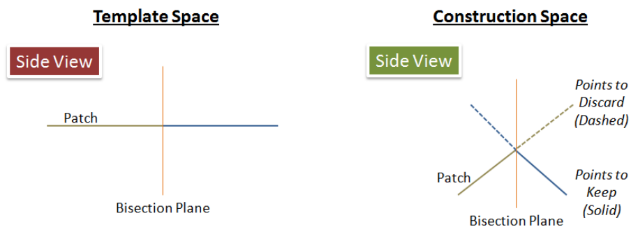
Fig. 47. Points from an inter-surface intersection caused by articulation can be removed by finding the bisection plane at the joint, and performing a simple spatial test to identify the points that lie on one side of this plane in template space and the opposite side in construction space.
