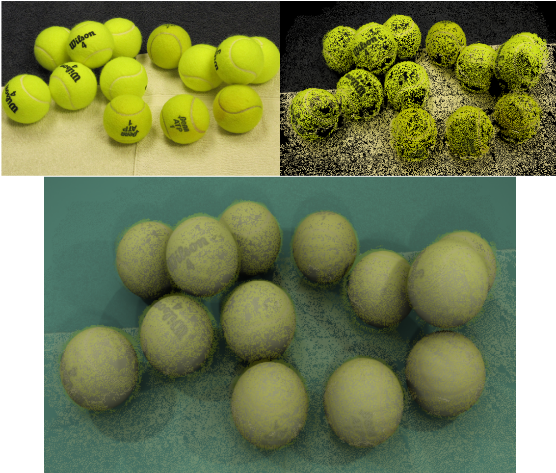
Fig. 31. A photo-based point cloud and corresponding set of reconstructed models (Example 9).
