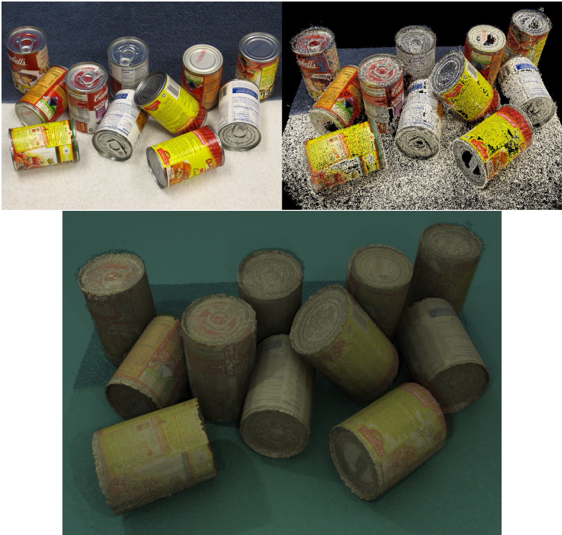
Fig. 33. A photo-based point cloud and corresponding set of reconstructed models (Example 11).
