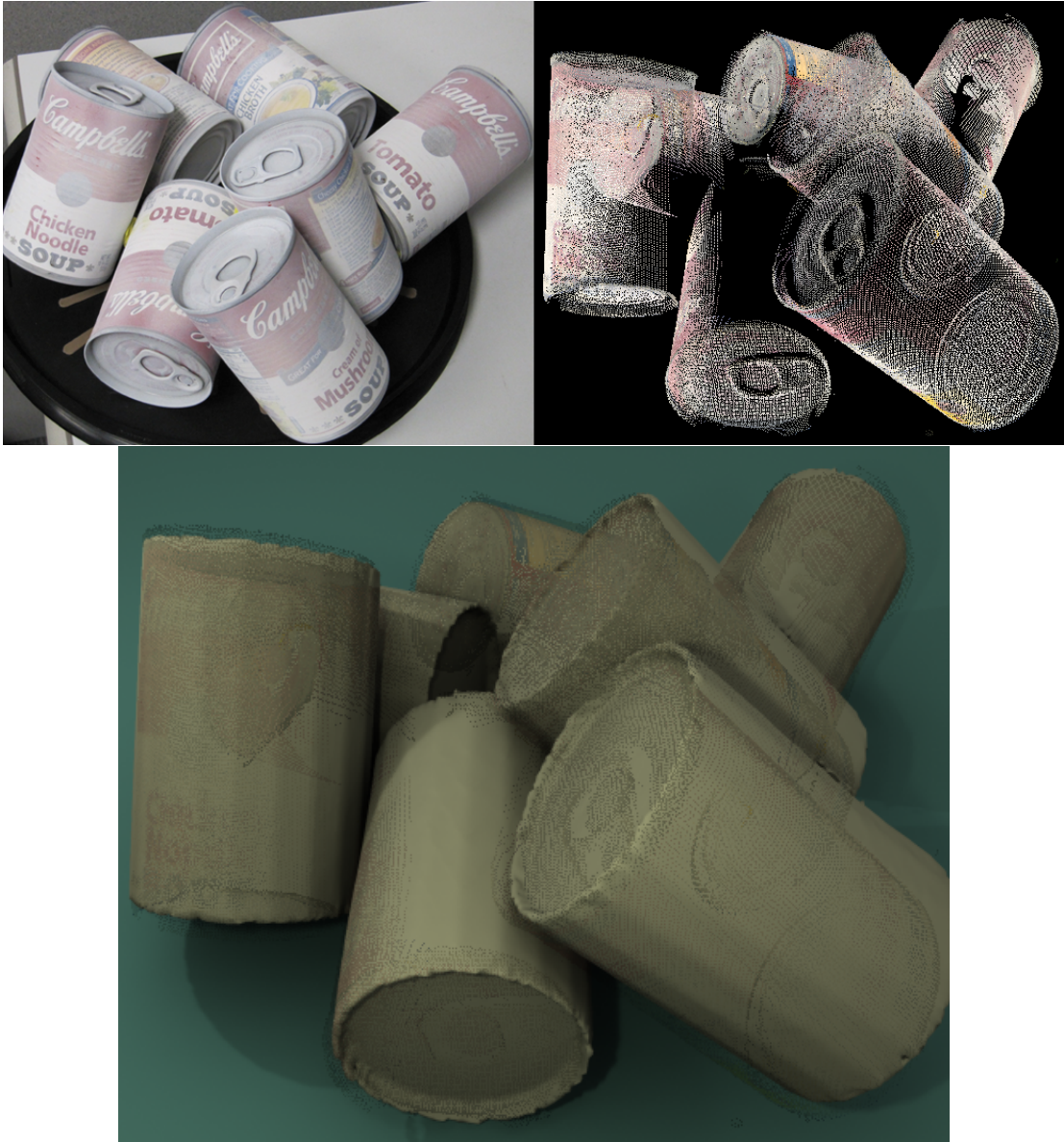
Fig. 30. A laser scan-based point cloud and corresponding set of reconstructed models (Example 8).
