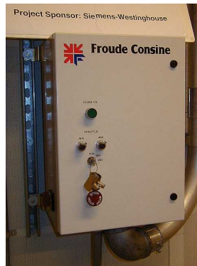
Fig. 88.: Power supply box for dynamometer
