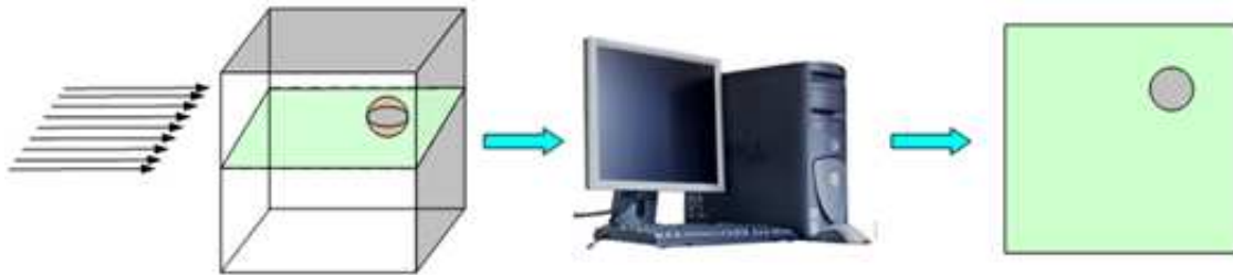
Fig. I.2: Sketch for traditional computer tomography (CT) procedure.
