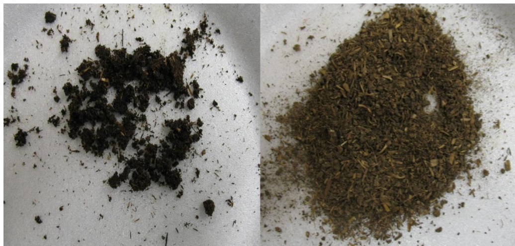
Fig. 34. Fuel color variation as it enters the reactor.
