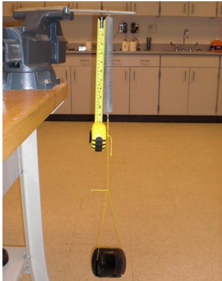
Fig. 11. Calibration procedure for the spring.
