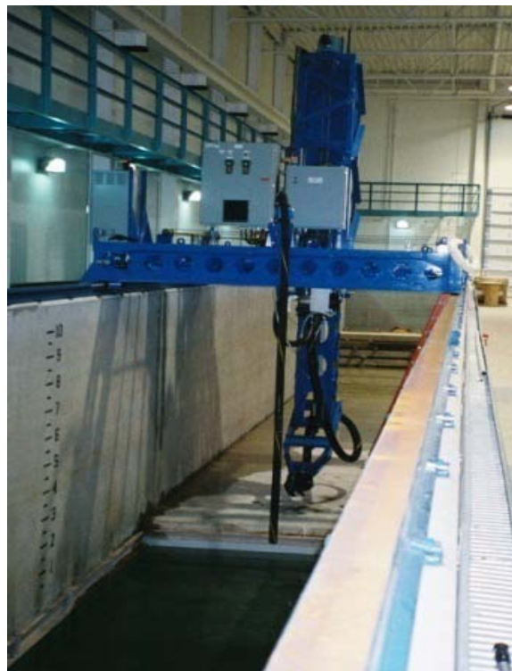
Fig. 4. Dredge/tow carriage and tank in front of sediment pit filled with water.
