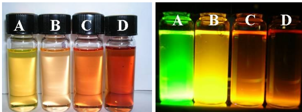
Figure 13. CdSe/ZnS QD's in chloroform as seen in ambient light (L) and under UV light (R).
