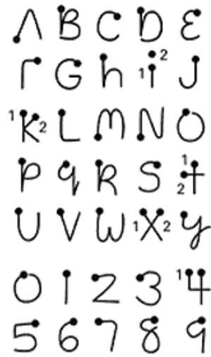
Fig. 11. Example gesture set from Graffiti. Some of these gestures may not be natural to the user and must be learned before interacting with the system.
