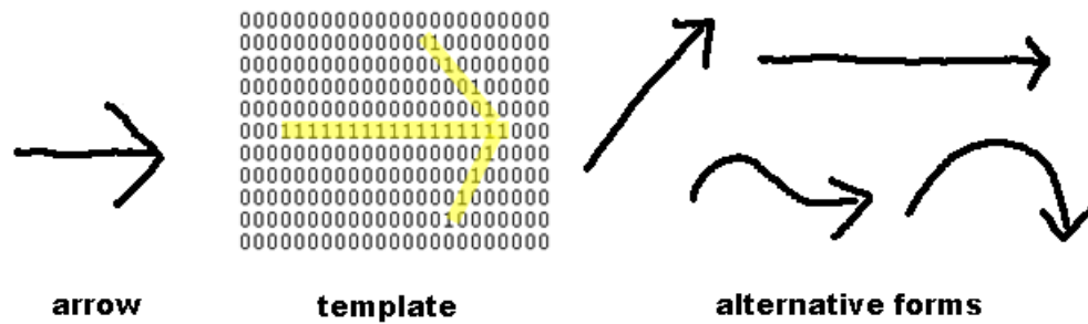
Fig. 14. Appearance-based methods typically use some form of template matching to perform recognition; however, alternative variations of the same symbol would require multiple templates.
