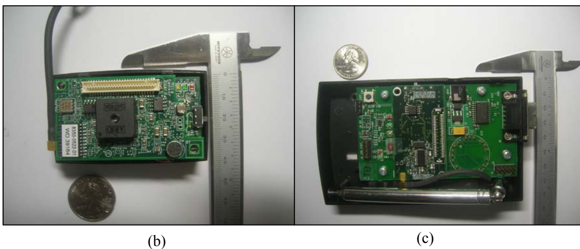
Figure 12. (a) Test set-up for a simply supported beam for including MICA 2 motes, base station, and lap-top computer, (b) MICA 2 mote, and (c) base station
