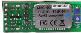
Fig. 3.4. Bluetooth integrated circuit. This device is the heart of the communication between the controller and the plant.
