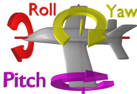
Fig. 2.1. Euler angles yaw \psi , pitch \theta and roll \phi .
