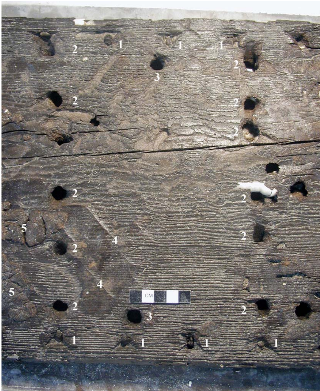
Fig. 4.16. Frame station on plank UM1, inboard face. (1) Tetrahedral notches and ligature holes with in situ wooden pegs. (2) Paired oblique frame lashing holes. (3) Treenail holes. (4) Preserved original surface and adze marks. (5) Remains of pine tar surface coating.
