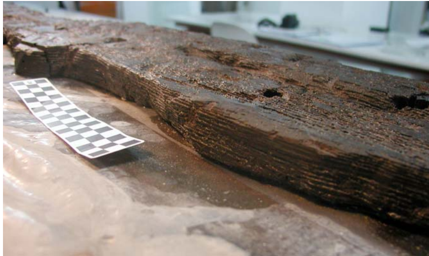
Fig. 2.5. Beveled edge of the curved scarf on plank UM1.
