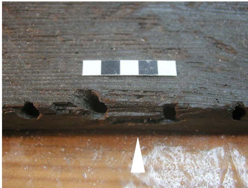
Fig. 2.16. Small mortise cut into the edge of plank UM5 between two ligature holes.
