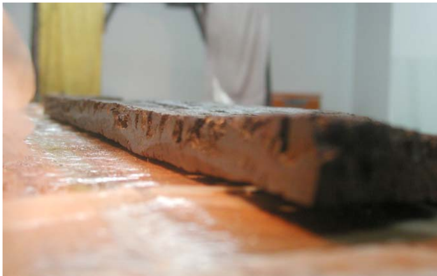
Fig. 2.15. Adzed edge of plank UM5.
