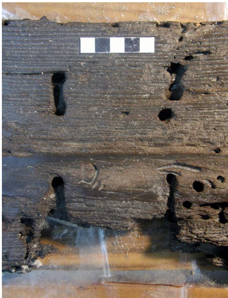
Fig. 4.17. Frame lashing holes on the outboard face of plank UM5. The lower holes of the two bottom sets are missing, but the grooves connecting them to their partner holes are mostly intact.
