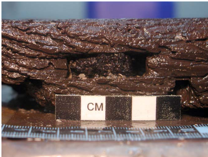
Fig. 2.9. Half-tenon preserved in its mortise in plank UM1.
