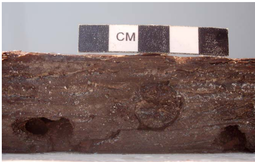
Fig. 2.18. Dowel in situ in the edge of plank UM6.
