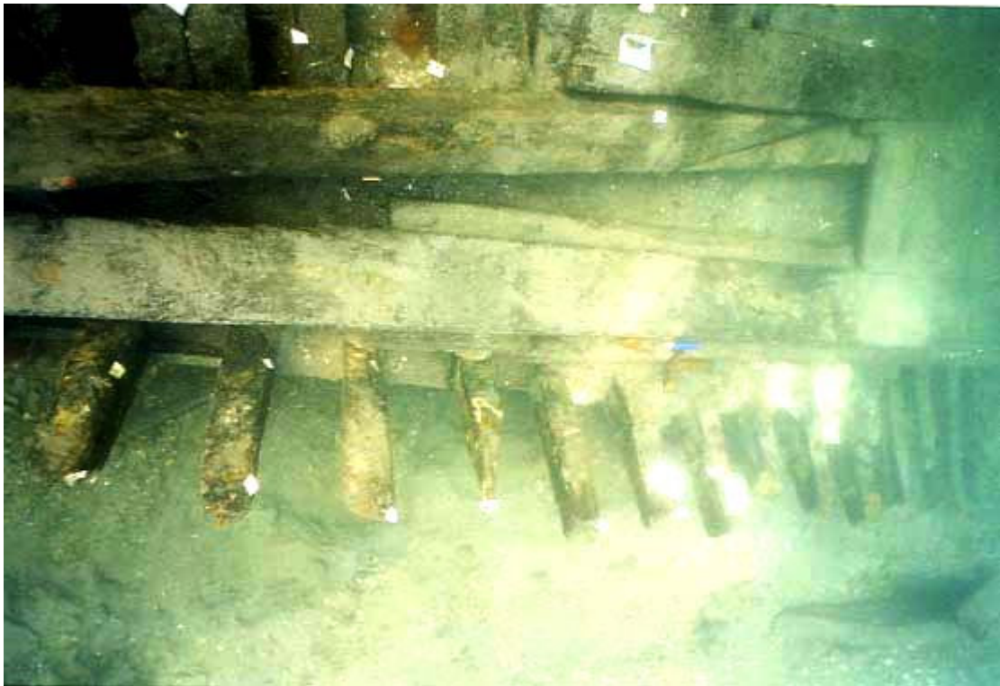
Fig. 20. The top of the keelson in the bow section. No trace of fasteners are observable. Photo: K. N. Batchvarov.
