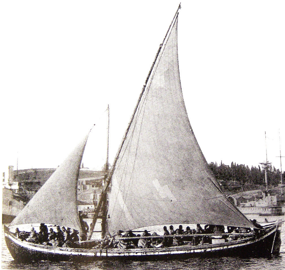
Fig. 61. A passenger alamana , with a stub mast and almost gunter-like lateen sail. Borgschultze incorrectly identifies the vessel as a mahone . 222 Note the difference in profile from fig. 62, which indeed is a mahone .
