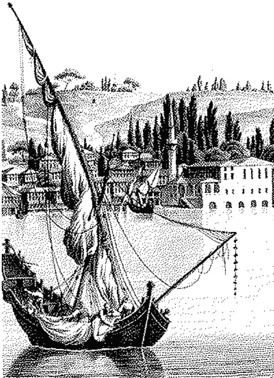
Fig. 53. A lateener with heavily raked mast. This vessel is probably very similar to the Kitten ship. Shrouds are set up with tackles. Detail from Melling, reprinted by Müller-Wiener in Plate 20.
