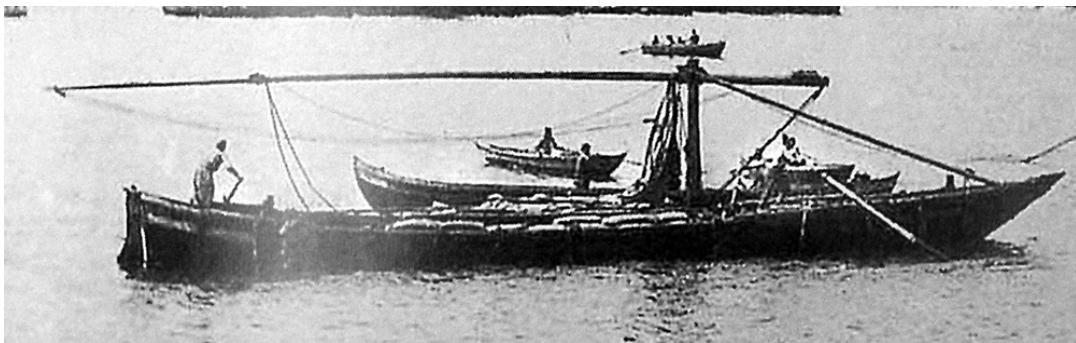
Fig. 62. A mahone with lowered yard for passing under bridges. Detail after a photo in Borgschultze.
