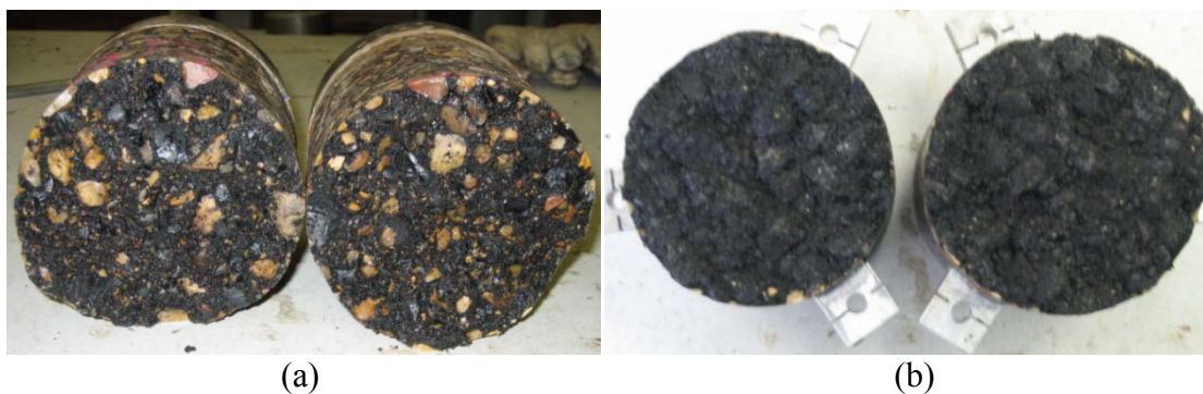
Figure 10-9. Test Specimens after Failure (a) Wet Condition, (b) Dry Condition.
