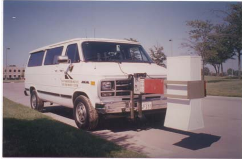
Figure 8-2. TTI GPR Equipment (Scullion, 2006).
