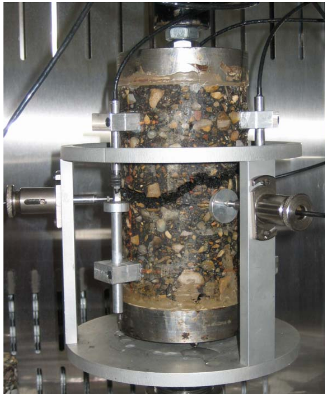
Figure 10-8. Test Sample after Failure inside the MTS Machine.
