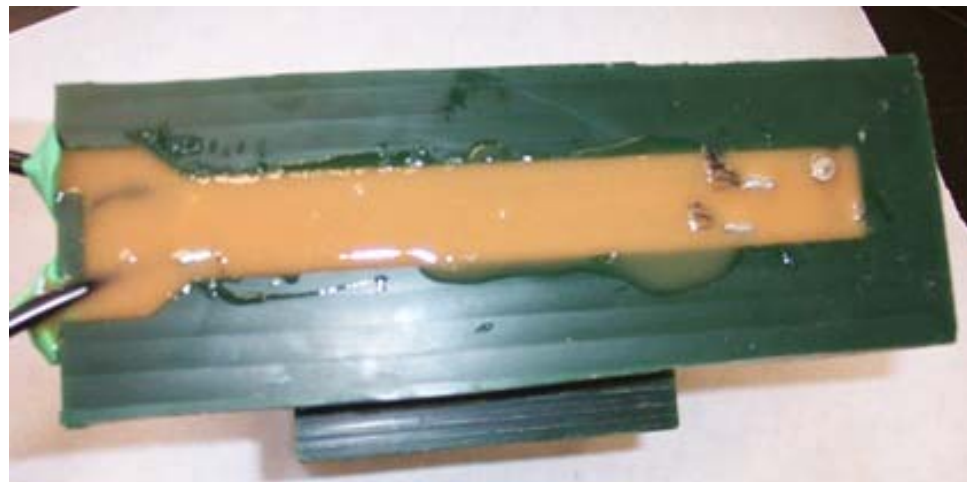
Figure 28. Fabricating a double embedded sheet.
