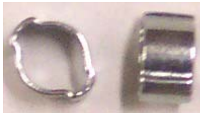
Figure 8. Zinc plated double pinch hose and tube clamp purchased from McMaster Carr.
