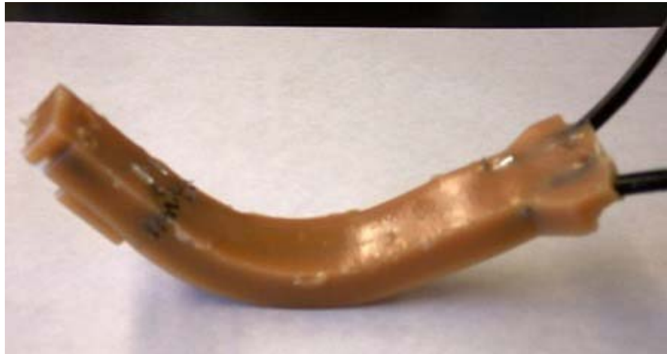
Figure 29. This double embedded muscle sheet shows that the muscles bend the sheet as they contract passively.
