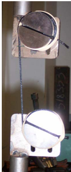
Figure 17. The braided polyethylene terephthalate mesh failure analysis per rope test.
