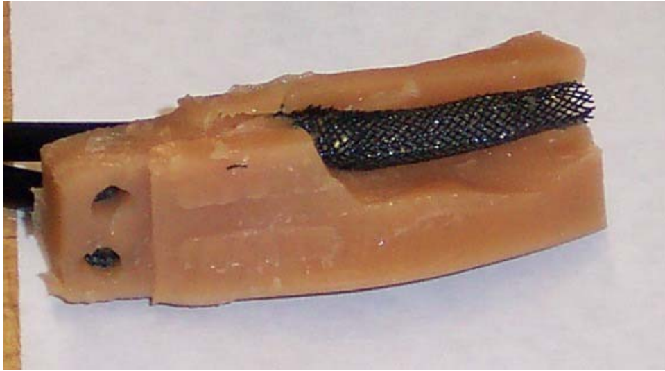
Figure 151. This picture illustrates that the muscle was not bonded to the polyurethane matrix. The elastomer matrix was cut open. The braid and inner latex tube have no matrix bonded to them.
