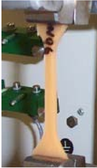
Figure 16. Testing procedure of the polyurethane dumbbell per ASTM standard.
