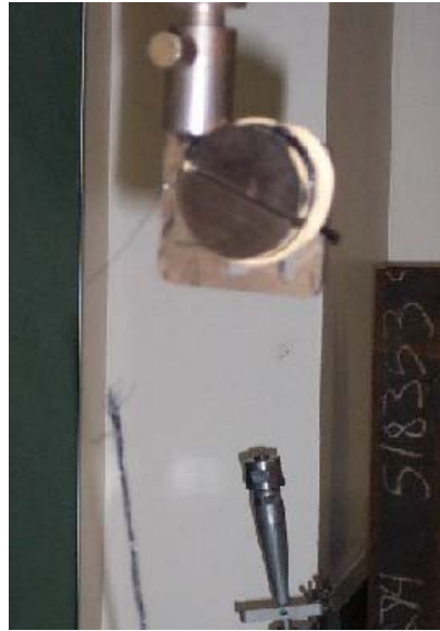
Figure 55. This picture represents a failed polyethylene terephthalate mesh sleeve using the rope test method.
