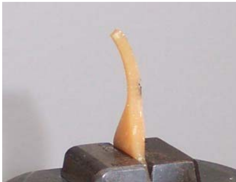
Figure 49. This picture represents the bottom half of one failed polyurethane dumbbell.
