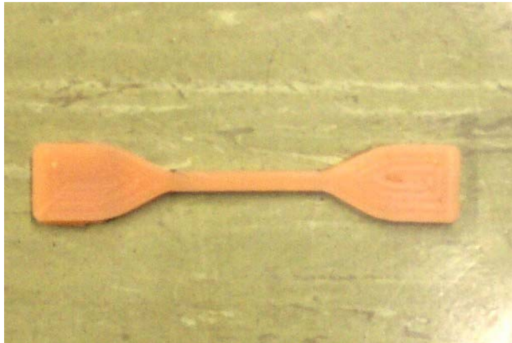
Figure 2. Elastomer matrix built into a dumbbell shape for testing.
