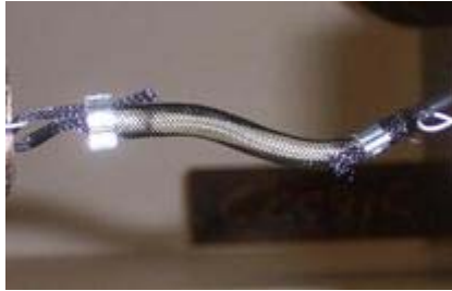
Figure 9. An example of a McKibben muscle built in-house.
