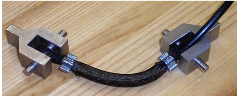
Figure 18. McKibben muscle installed into the holding fixture.
