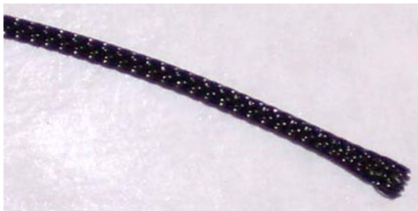
Figure 4. Braided PET mesh sleeve purchased from McMaster Carr.
