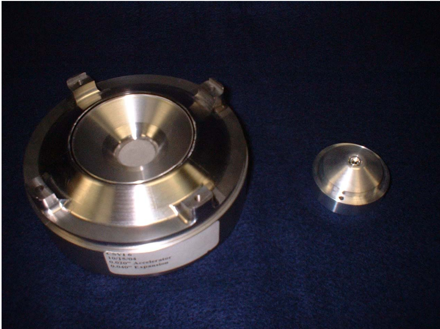
Figure 3: Inside of first and second stage CSVI units.
