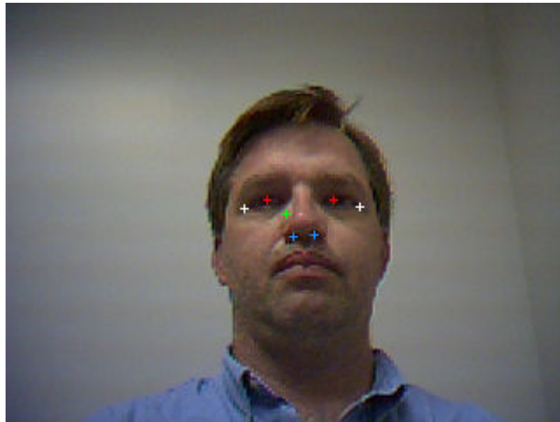
Fig. 9 Features located using skin color and geometric constraints.
