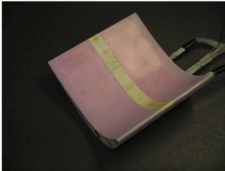
Figure 5.3 Blade for surface pressure measurements with 48 static pressure taps and a binary pressure sensitive paint (PSP)
