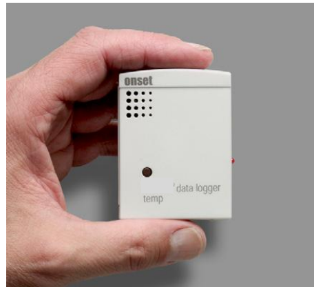
Figure 3: Mini-Data logger used to assess the building performance.
