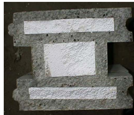
Figure 2. Photo of bazelt block With three lines thermal insulation
