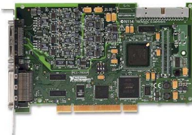
Fig. 3. National Instrument's PCI-7831R FPGA card. The FPGA allows for high frequency loop rates.
