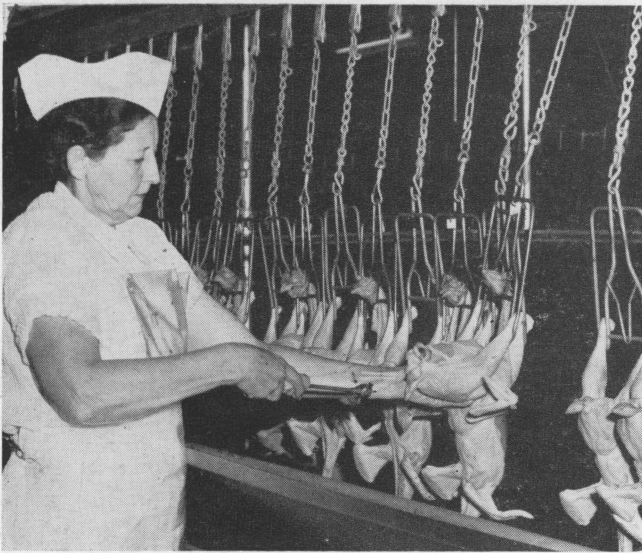
Figure 9. Lungs can be removed from 660 to 1,200 birds per hour with a Lynn lung remover.
