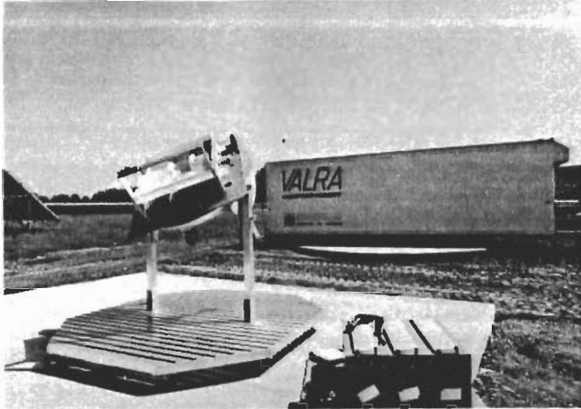
Fig. 6 Rotating Test Building and Heliodon
