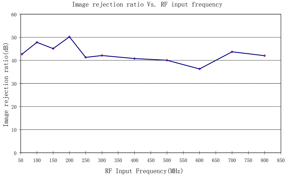
Fig. 2.24. Measured image rejection ratio vs. frequency
