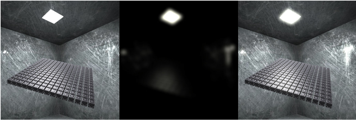
Fig. 16. Bloom Effect. Without bloom effect (left), HDR Mask (middle), and with bloom effect (right).
