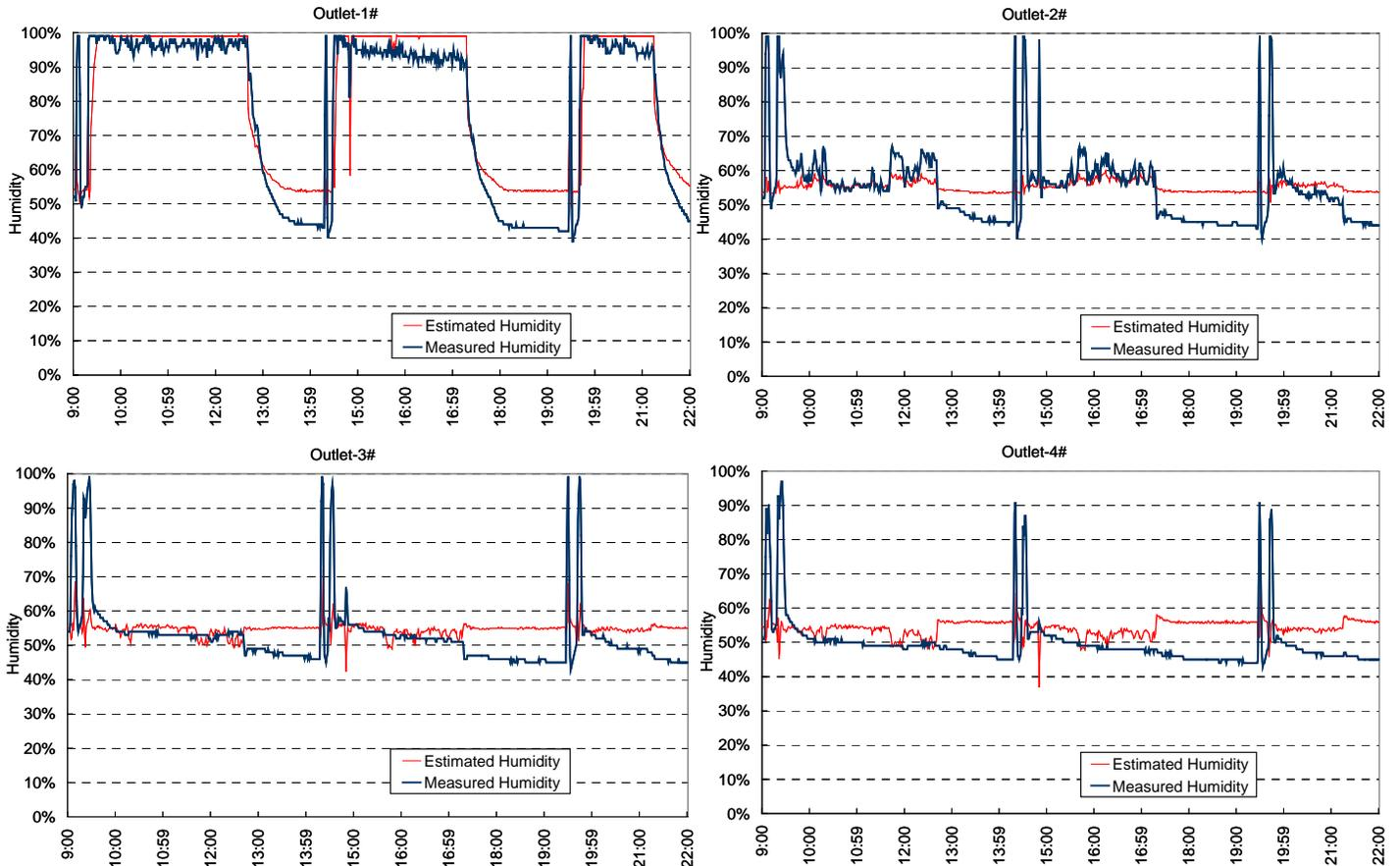
Figure 6. Estimated and measured outlet air humidity at four outlets
