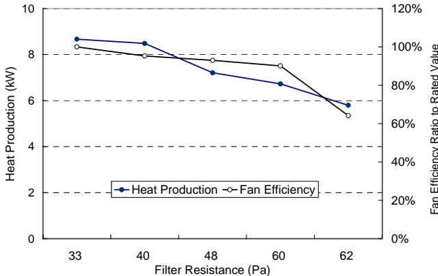
Figure 1. Heat production and fan efficiency vs. filter resistance
