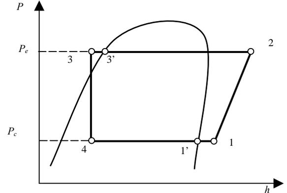
Figure 2. Refrigeration cycle state points
