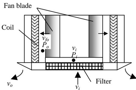
Figure 3. Measurement points in a typical cassette-shape indoor unit
