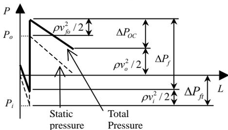
Figure 4. Pressure curve of indoor units
