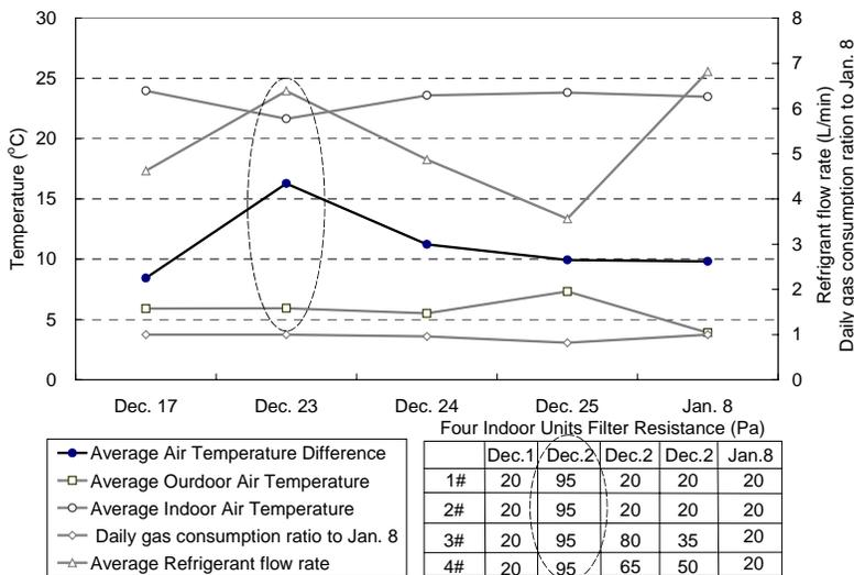
Figure 7. An air-conditioner's performance vs. filter resistance
