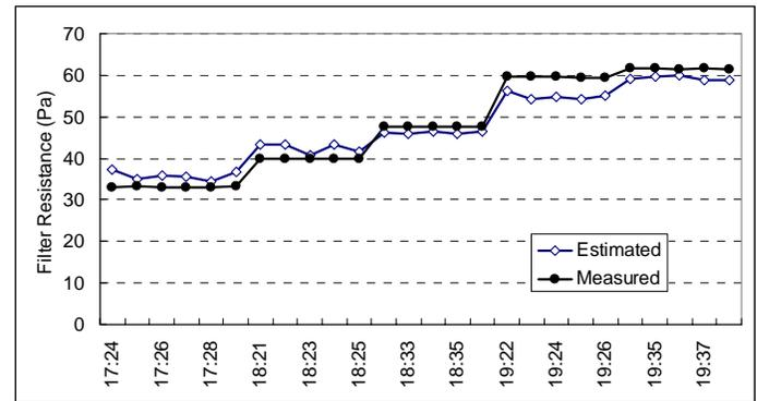
Figure 11. Validation results of estimating using fan power consumption
