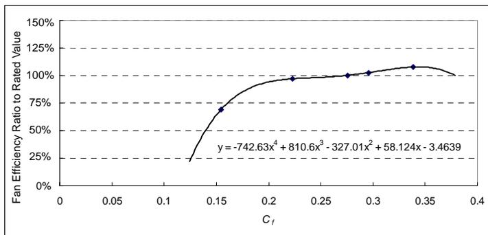
Figure 9. Coefficients fitting results of indoor unit fan
