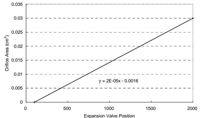
Figure 10. Expansion valve orifice area vs. controller demand
