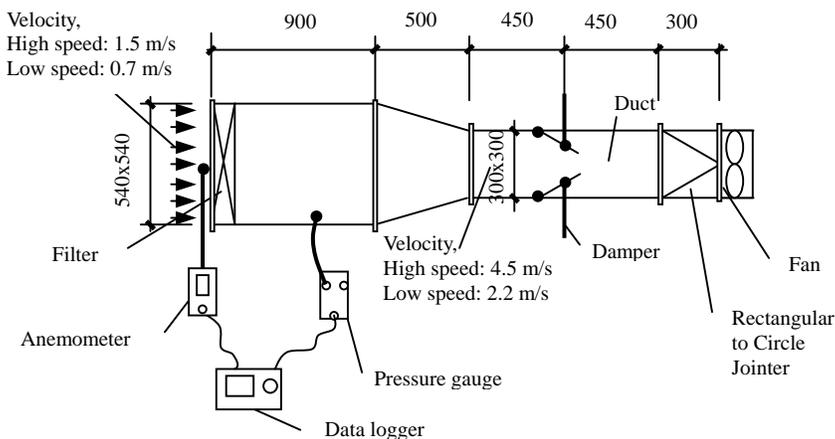
Figure 8. Ducts and instruments for making filters having different resistance
