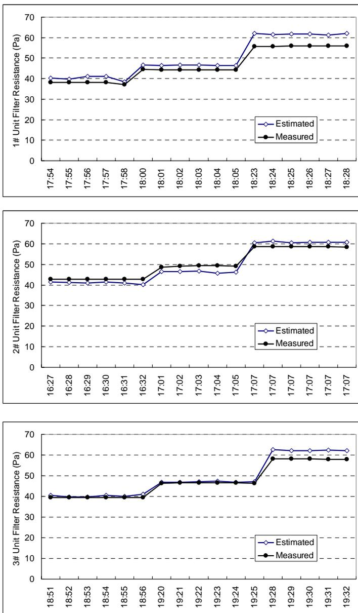
Figure 13. Filter resistance estimation results of three other indoor units
