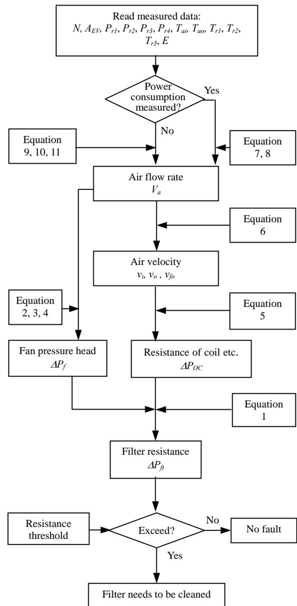
Figure 14. Flow chart of model-based automated commissioning for filters in air-conditioners
