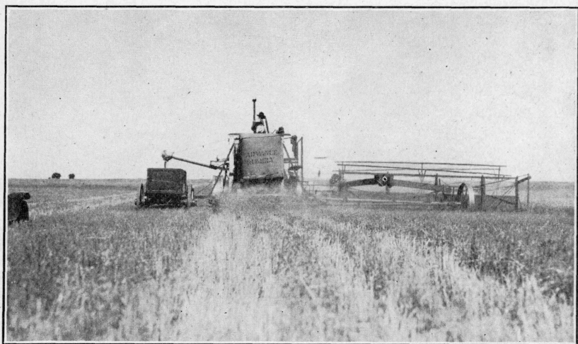
Figure 3.—A twenty-foot combine in operation. A machine of this size will harvest and thresh 50 acres per day and is well adapted to large-scale wheat farming as found in the Texas High Plains Section.
