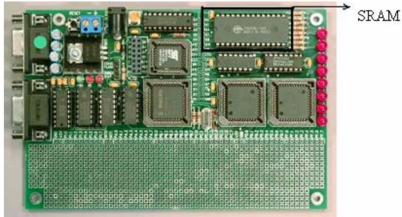
Figure 3.1 Layout of the board and SRAM used for experiments.
