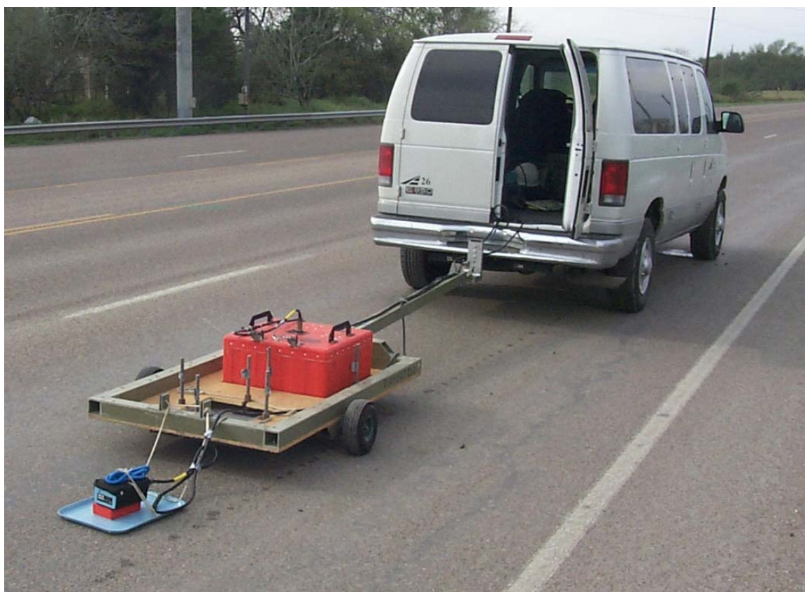
FIGURE 3 Ground-Coupled GSSI Antennas Used on the Second GPR Survey.
