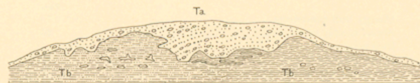
FIGURE 2.—Tertiary deposits in railroad cut one-quarter mile west of Granite Canyon, Wyoming; looking north. Length, 100 feet; height, 30 feet. Ta, Arikaree formation; Tb, Brule clay. Granite porphyry underlies the section shown.
