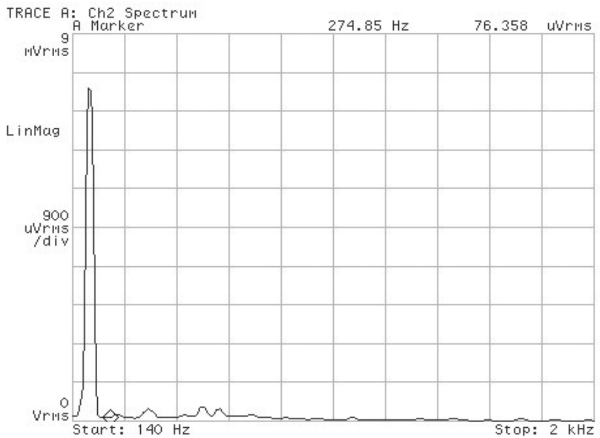
Fig. 53. The signal spectrum of the output of filter #5 with 50mVpp and 470Hz sinusoidal input.
